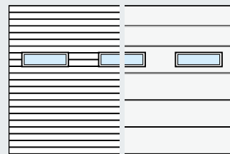
With compound window type D Door section heights: 500, 625, 750 mm
