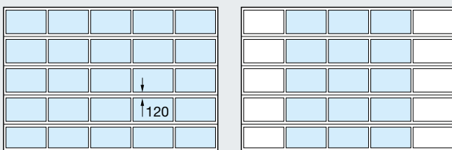
Available fully glazed or with an individual arrangement of the glass and panel infills
