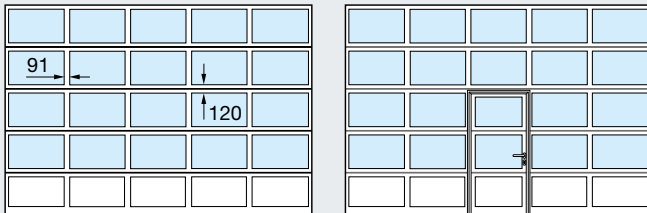
As standard with a 91-mm rail extrusion for doors from 5510 mm wide
