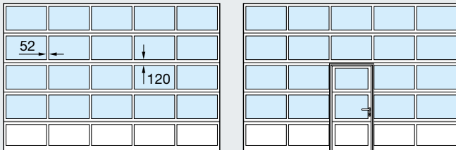
With 52-mm rail extrusion (on request with 91-mm rail extrusion) for doors up to 5500 mm wide
