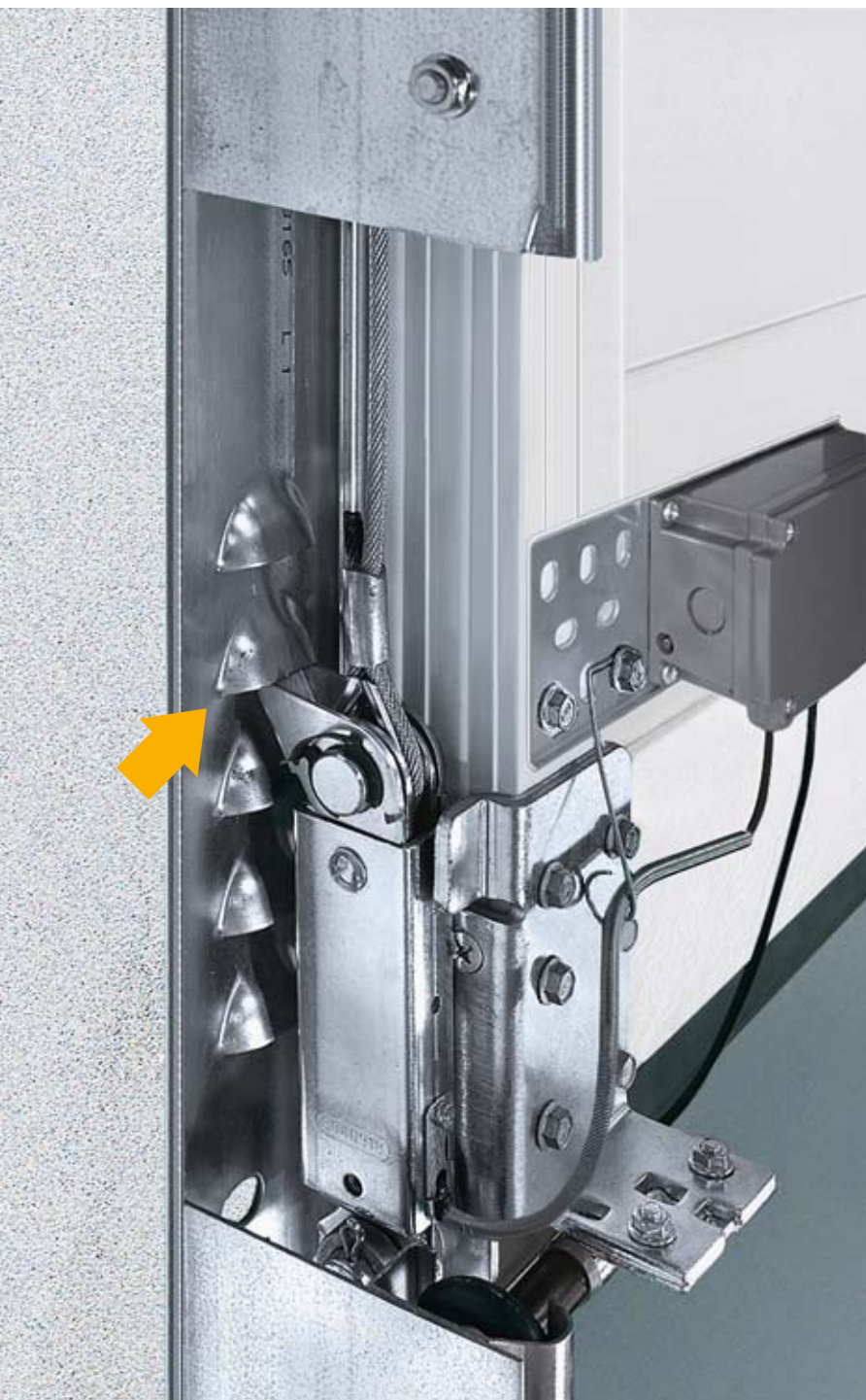
The locking hook of the arrestor kit automatically latches if the door is forced upwards.
